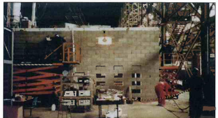
Figure 10 BRE/FRS Full-Scale Test Rig (side view)
